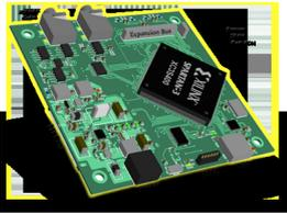
Mimzy (beta code-name) is an FPGA development board I have designed for a few projects I am planning and will also be part of the [Your First CPU](#) project for implementing and testing the custom soft processor core and ucLinux. Features include 8Mb Flash, 32MB SRAM, sound codec, SD Slot and USB. I have completed the schematics and PCB routing but I have not yet tested the design beyond some spice modeling. Some aspects of the design may still change.
